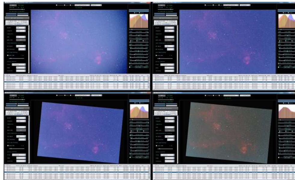
Figure 8: 4 images modes of light frame with an exposure of the Heart Nebula Top Left: linear(l) Top Right: l-calibrated Bottom Left: l-c-registered Bottom Right: l-c-r-normalised
